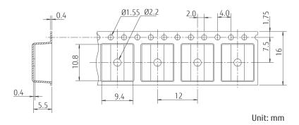
Relays are sold in 1000 pieces per box. Minimum order quantity is 1000 pieces for tube and tape & reel packing.
